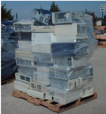
**✘** Load is not 100% covered in wrapping and pallet is not secured to load.
