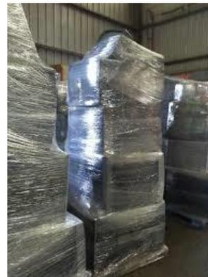
**✔** Pallet is wrapped with at least 3 layers. Load is 100% covered in wrapping and load weight spread across covers entire pallet.
