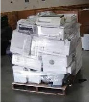
**✘** Items have not been wrapped in at least 3 layers of wrapping. Items are overhanging the side of the pallet and have not been secured to the base with strapping.
