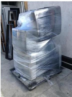
**✘** Heaviest items have not been stacked on the bottom. Items are overhanging the side of the pallet and have not been secured to the base with strapping.
